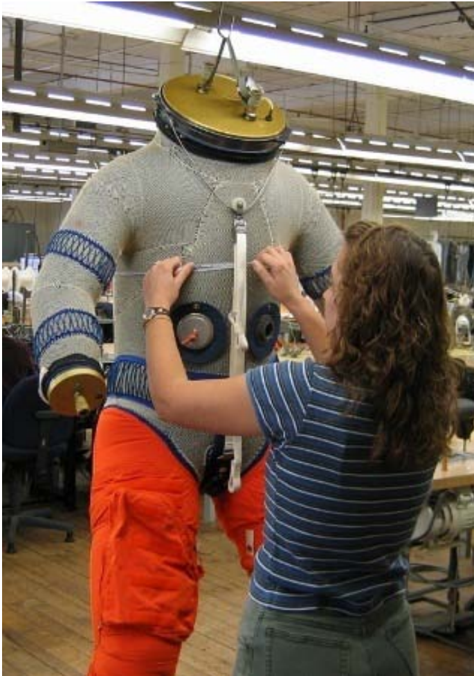
Above - ACES Continued the X-15/Gemini-Developed Linknet Restraint System in the Upper Torso (Courtesy DCC)
