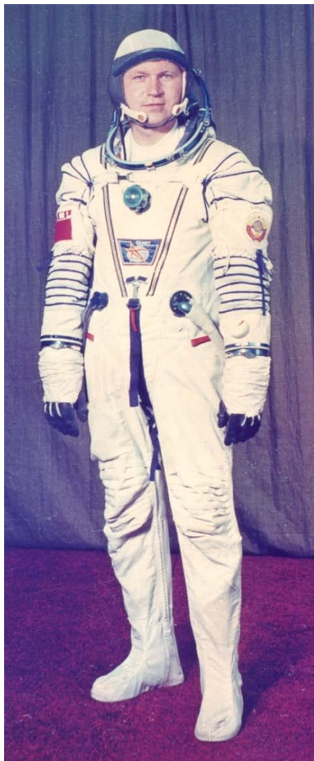
SOKOL-KV-2, The Current Russian LEA Spacesuit (Courtesy Gary Harris)
