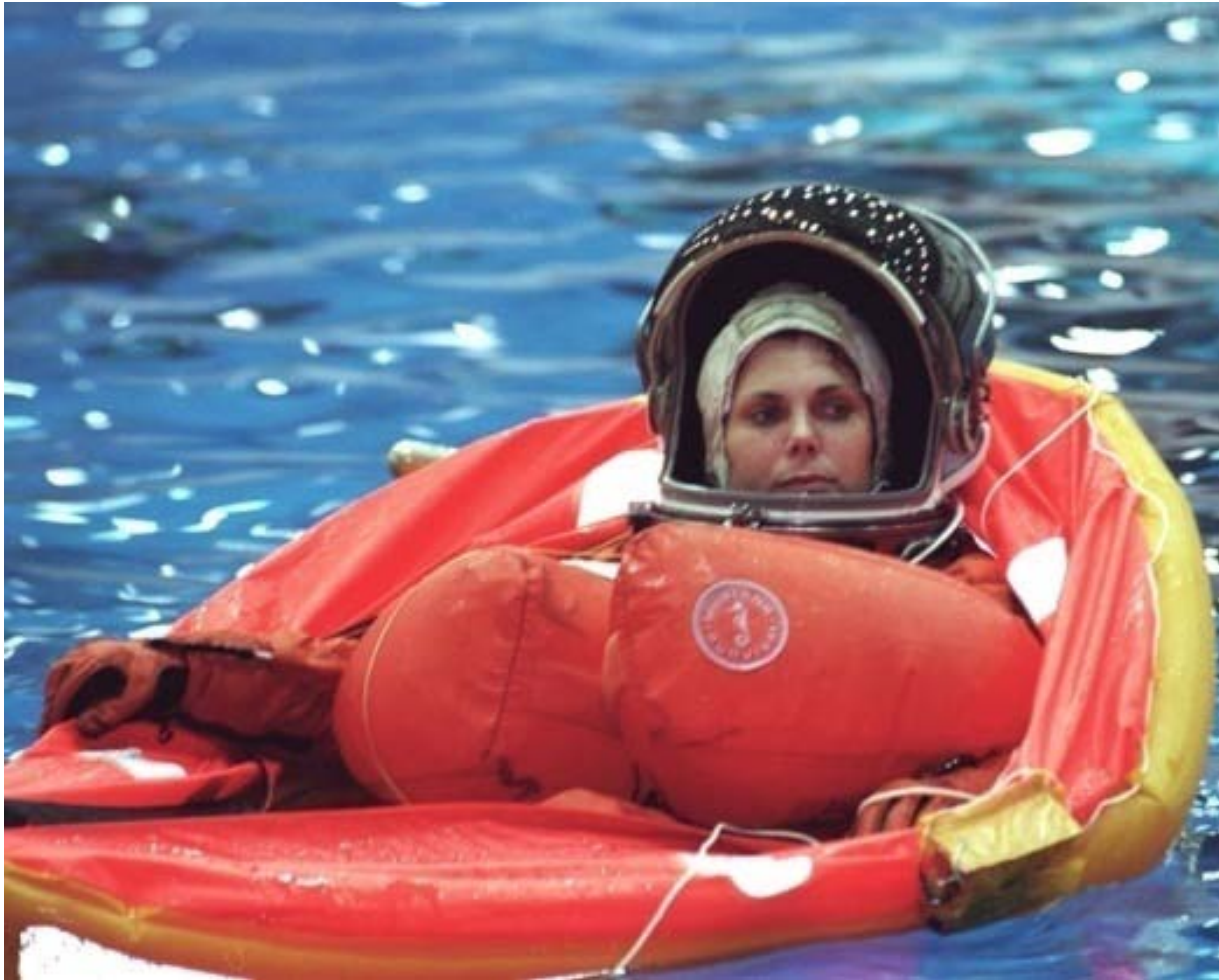
The ACES Pressure Garment had an Integrated "Mae West" Flootation System and Carried a Raft (Both Shown Deployed)
